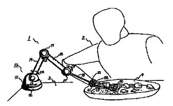
ABSTRACT: PROBLEM TO BE SOLVED: To simplify the constitution, and effectively assist everyday life or the like such as a manual work by a method wherein at a free end of this assisting device, an appliance which is fitted on an upper limb of a person to be assisted, is provided, and the track of the free end is controlled based on force information of the person to be assisted, which is applied to the appliance, and the motion of the upper limb is assisted.
